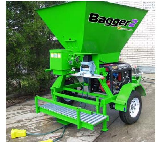
Place your bag over the bag holders, press the pedal for loading material into the bag. Once it has reached the desired timed amount the conveyor will stop.
