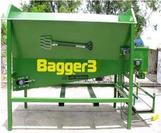
This smart little Bagger 2 unit holds approximately 2 cubic meters of material ready for bagging and can be used for compost, bark chips, dry sand, small pebbles etc.
