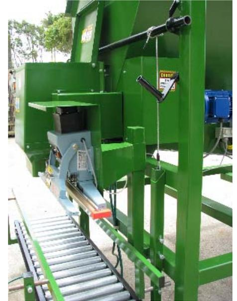
Place the top of the plastic bag into the opening on the sealing unit being careful not to get your fingers in the road. Place your foot on the other pedal which operates the closing of the sealing unit.
